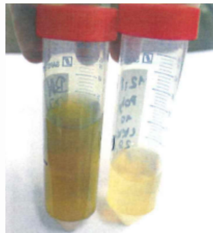
Fig. 1: Right hand side: end-product obtained by using optimized DMC complexes as catalysts
